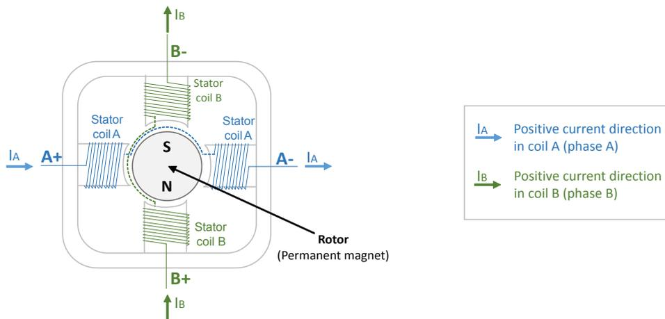
The current flowing in one phase generates a magnetic field. If both phases are energized, the stator magnetic field is the combination of the two perpendicular fields generated by the two phases, as in [Figure 2](#). The rotor moves in order to align its own magnetic field with the stator one.
