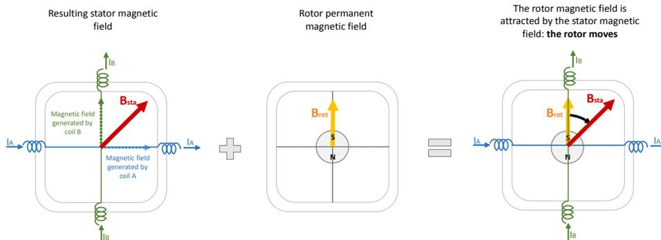
Changing the direction of the currents in the phases, it is possible to align the rotor along the different steps. Therefore, driving the phase currents with a proper sequence, it is possible to move the motor shaft step by step.
