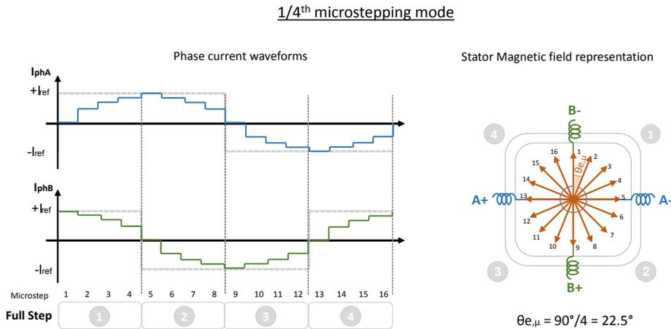
The increasing of the microstepping mode allows to have smoother sinewaves and a small angle between the microsteps. A smooth and constant rotation of the stator magnetic field results in a smoother movement of the motor shaft. For lower microstepping modes, the quantization can be seen on the sinewaves; conversely, using the maximum resolution (256 microsteps), the current sinewaves are very smooth.
