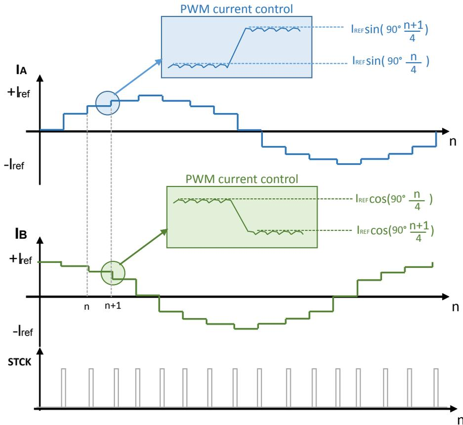
It can be seen from **Figure 7** that the maximum reference current on one phase corresponds to the zero current in the other phase. The resulting current given by the combination of the two currents is equal to  $I_{REF}$ ; this is true in all microstepping modes. While in full step mode, both currents are equal to  $I_{REF}$ , so their combination is  $\sqrt{2} I_{REF}$  as described in the **Section 1.1**.
