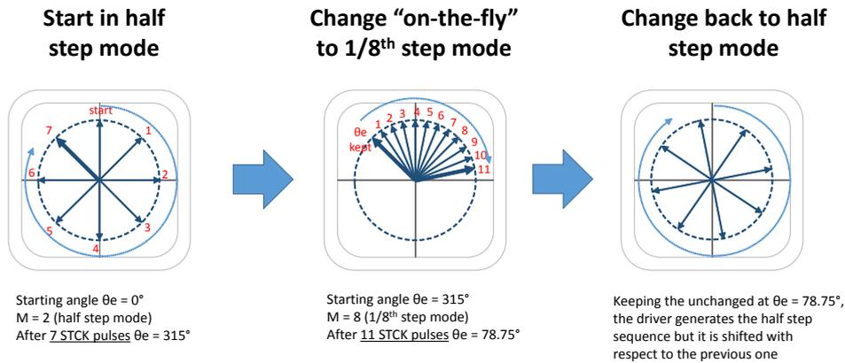
In order to maintain the sequence unchanged when changing from one resolution to another, the mode switching must occur at one electrical angle available in the lower microstepping mode. In the example of Figure 10, when changing from 1/8<sup>th</sup> ( $M=8$ ) to half step mode ( $M=2$ ), the change must occur at  $\theta_e$  multiple of  $45^\circ$  (that is  $90^\circ/M$ ).
