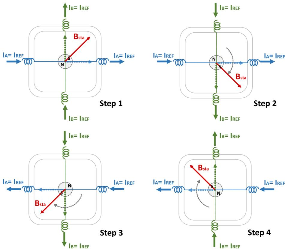
Repeating the full-step sequence results in a continuous rotation of the motor. In the STSPIN820, every pulse on the step clock pin (STCK) triggers a change from one step to another. The direction in which the sequence is performed (so the direction of the rotation) is selected by the DIR pin.
